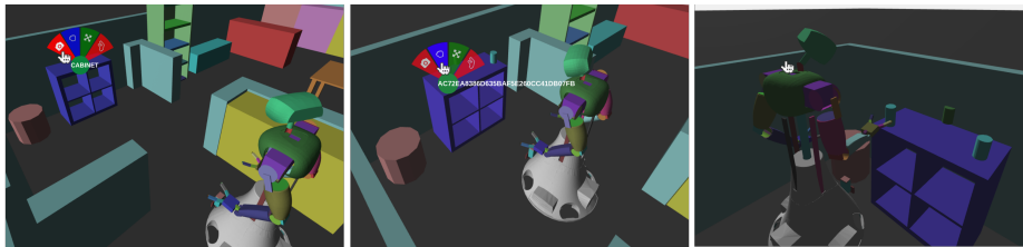
Fig. 6. Illustration of the 3D scene of the WebGUI with AMIGO. User can long-press objects to open a menu from which actions on the object can be triggered
