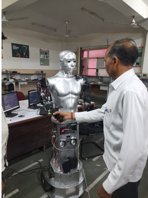
Fig. 2. Anushka, the robot without its clothing, performing a hand-shake on detecting a stranger.
