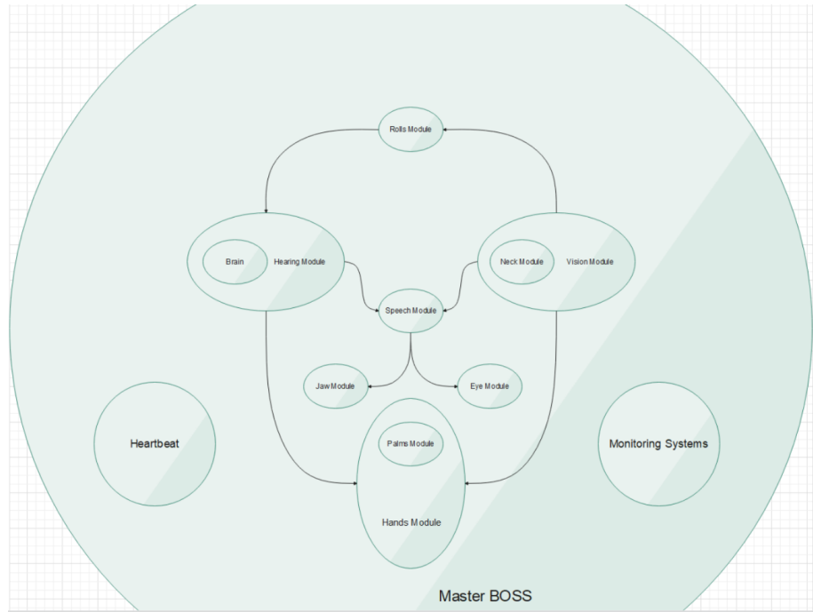
Fig. 1. The BOSS module receives sensing data from all the input modules and smartly decides which output module to command, automatically prioritizing tasks in a background thread.
