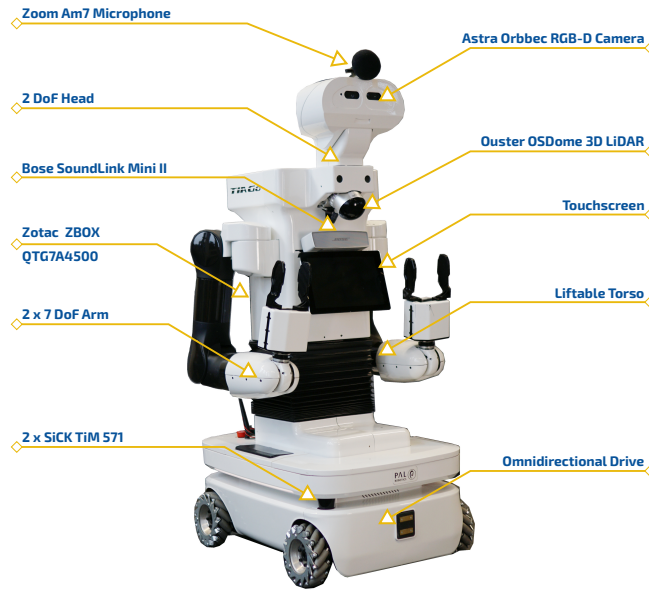
Fig. 2: TIAGo++ omnidirectional robot platform.
