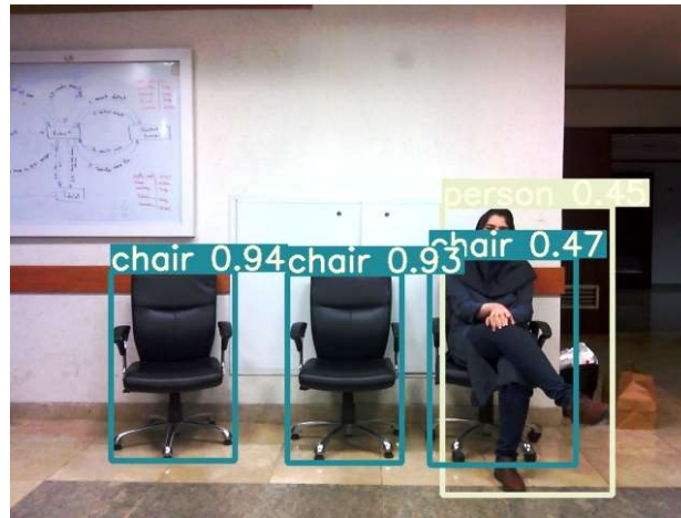
Fig. 4: detecting empty seats in the video stream received from Pepper's bottom camera
